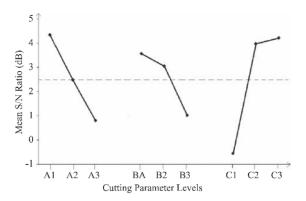
Fig: 2. S/n ratio graph for surface roughness
