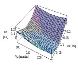
**Fig: 7.** Roughness surface variation with cutting speed and flank wear
