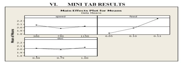
Effect of Turning Parameters on Surface Roughness
